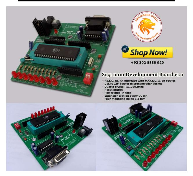
With this board you can develop and prototype with any of 8051 40 pin microcontrollers. The RS232 driver on board allows easy connection with PC or other embedded hardware. The board have status LEDs. The board can be powered DC power supply adapters 5V or 12V / 1 Amp.
